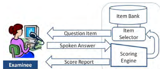
図 3 SJ-CAT automated speaking test system.
